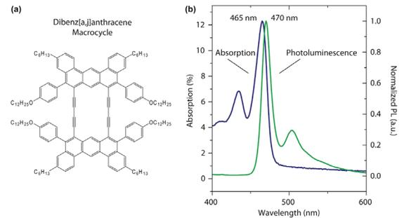
**FIGURE 1:** (a) Chemical structure of dibenz[*a,j*]anthracene-based macrocycle. (b) Optical absorption and photoluminescence spectra from a thin film prepared by spin-coating the compound onto a glass substrate. Thin film roughness of less than 1 nm was observed in AFM.
